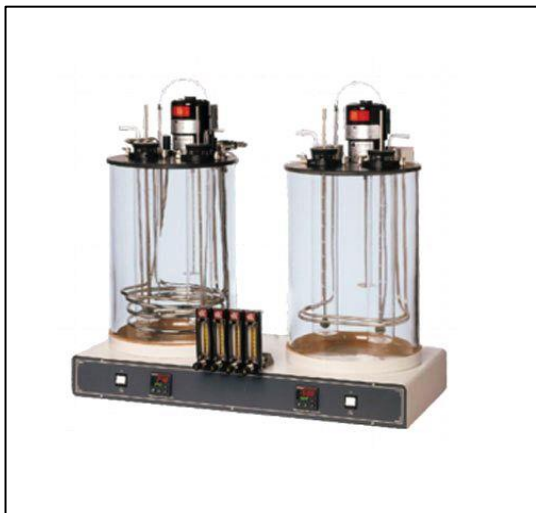
Figure 10 Foaming test apparatus
